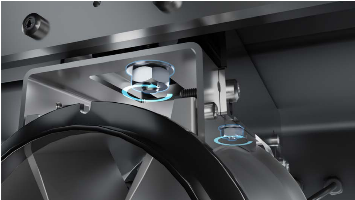
9. Tighten the bracket to the niche Secure the bracket to the niche by tightening the nuts. The turbine is now set to the correct base height and completely fixed mounted.
