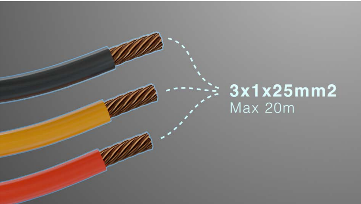
2. Choose your cable Use 3x1x25mm2 cable to a maximum cable length of 20 meter (total maximal 25 meter inclusive existing cable).
