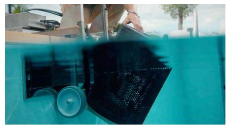
2. Unclip the rotating bracket (with EVAstream) on both sides and place it upright. Lower the EVAstream Move into the water.
