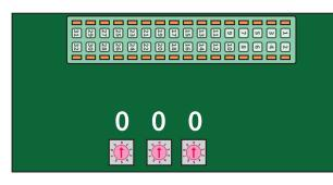
Setting the ECA Print: Set the Rotary switches at <u>000</u> (Master mode)
