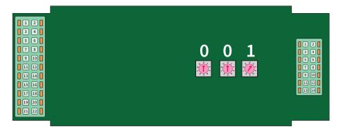
Setting the Control Print: Set the Rotary switches at <u>001</u> (Slave mode)
